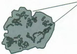
Hot metal is drawn into the irregular fissures of the porous **DegasCarb™** surface
